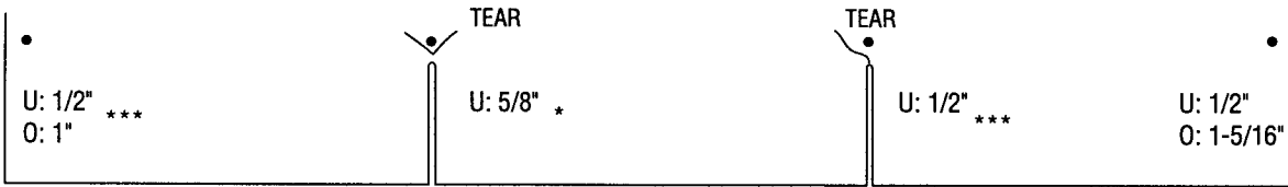
B2 H1 35° RUN 117 DAMAGE INDEX: 16 LONG DURATION
